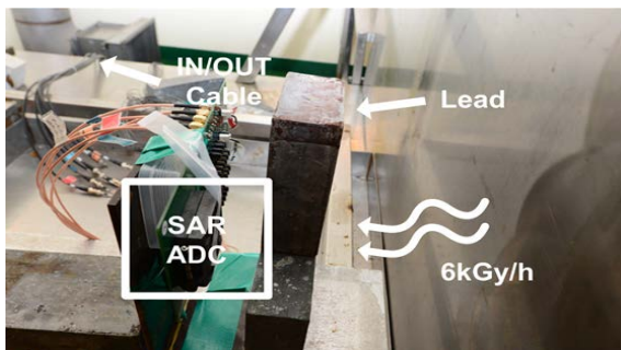
Figure 13. Chip test setup in the high-level radiation facility
